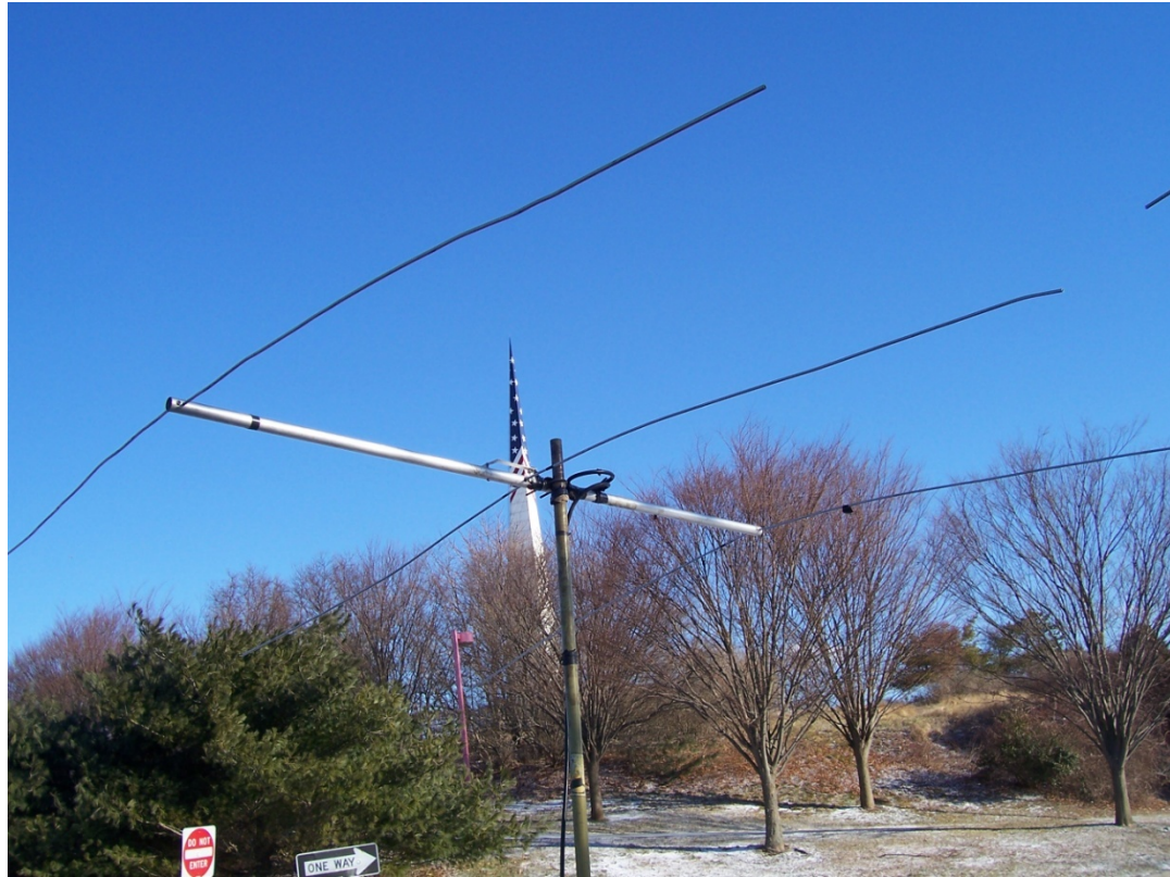
Three element Six Meter Yagi at portable location for January VHF Contest on hill 250 feet ASL in Central Long Island
